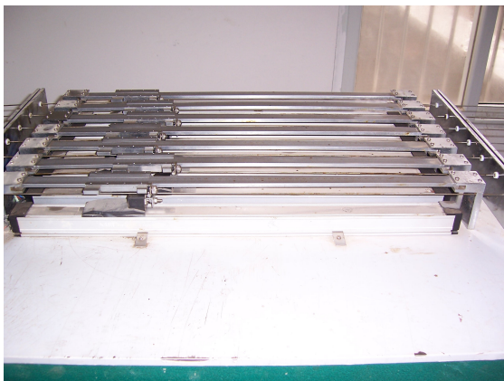
Figure 3: Interior wire extensometer.
